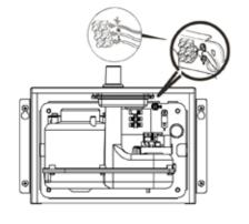
6. Mount unit cabinet to the wall. Insert power cord through the inlet hole located in the back of the cabinet, or through the premade opening at the bottom of the cabinet. Connect power cord to hand dryer. It may be necessary to remove a plate to push the cord through.
